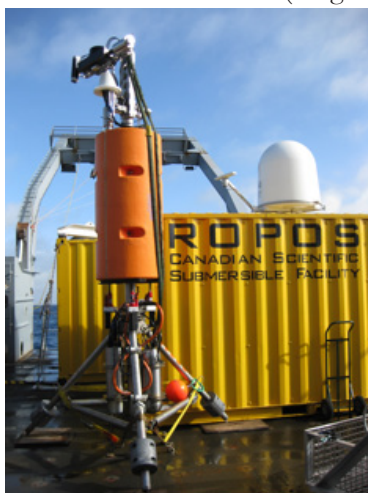
Figure 1: COVIS on deck of R/V Thomson. COVIS is 4 meters high with the sonar heads and orientation mechanisms on top, syntactic foam around the middle (orange), and sonar electronics in pressure housings between tripod legs.
