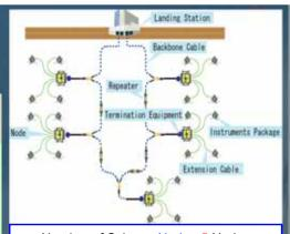
Number of Science Node : 5 Nodes Number of User Interface : 8 ports / Node Power Distribution : 30 W / Port Data Transmission : 50 Mbit / s / Port Precise Timing Control : < 1µsec
